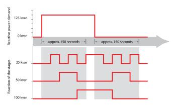
Power factor correction as our grandfathers knew it: the classical reactive power control relay using contactors to switch capacitor stages of different sizes in and out in a progressive sequence. It requires some 30 seconds per switching step until the target power factor is achieved.
