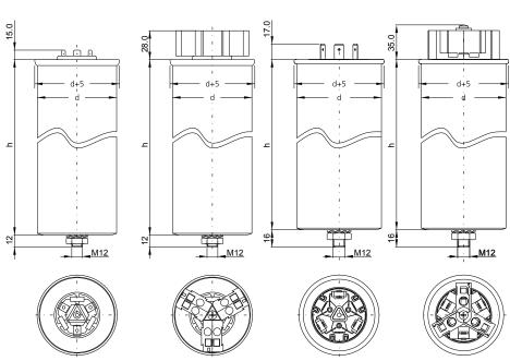
Capacitors with  $d = 60/70 \,\text{mm}$ for connection with flat cable plug 6.3×0.8 mm
