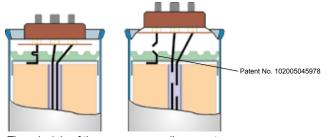
The principle of the overpressure disconnector
