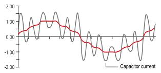
If, for example, the 11th harmonic is present with 8% of the rated network voltage, the r.m.s. value of the rated voltage is only increased by some 0.3%, but the current in the capacitors will exceed its rated value by 33%. It becomes clear that the ability of a capacitor to withstand excessive current is significantly greater than the ability to withstand excessive voltage.
